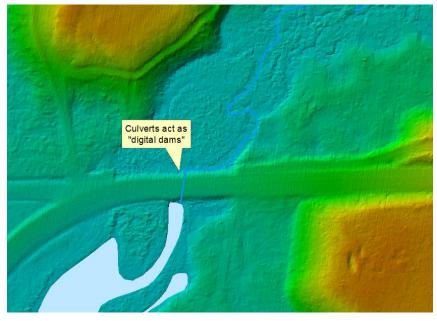
models require DEMs to be modifed with information about culverts, storm sewers, streams and ditches in order to remove these digital dams. This modification process is known as hydrologic DEM conditioning.
